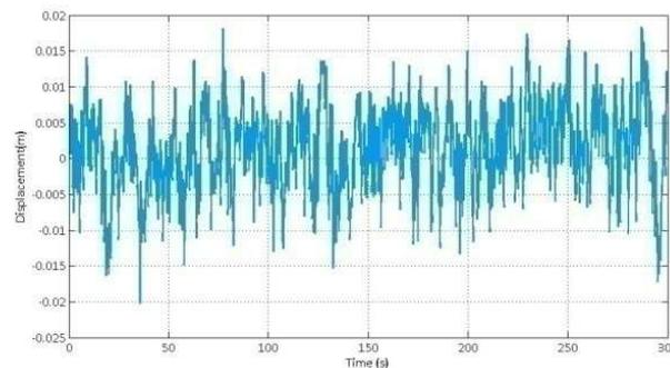
**Figure 9: QFRCo Sprung Mass Displacement: Randomc60**
