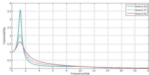
Figure 8: QFRCo Sprung Mass Transmissibility: Effect of Damping Coefficient
