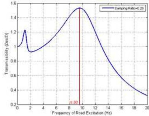
**Figure 3: QFRCo Sprung Mass Transmissibility    Figure 4: QFRCo Unsprung Mass Transmissibility**
