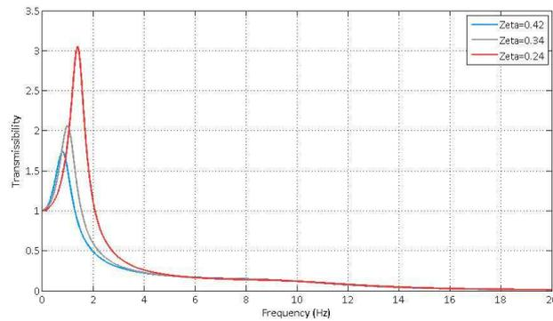
Figure 7: QFRCo Sprung Mass Transmissibility: Effect of Spring Stiffness
