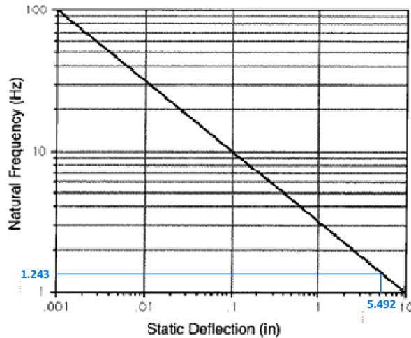
**Figure 5: QFRCo Suspension Static Deflection on Nomograms**
