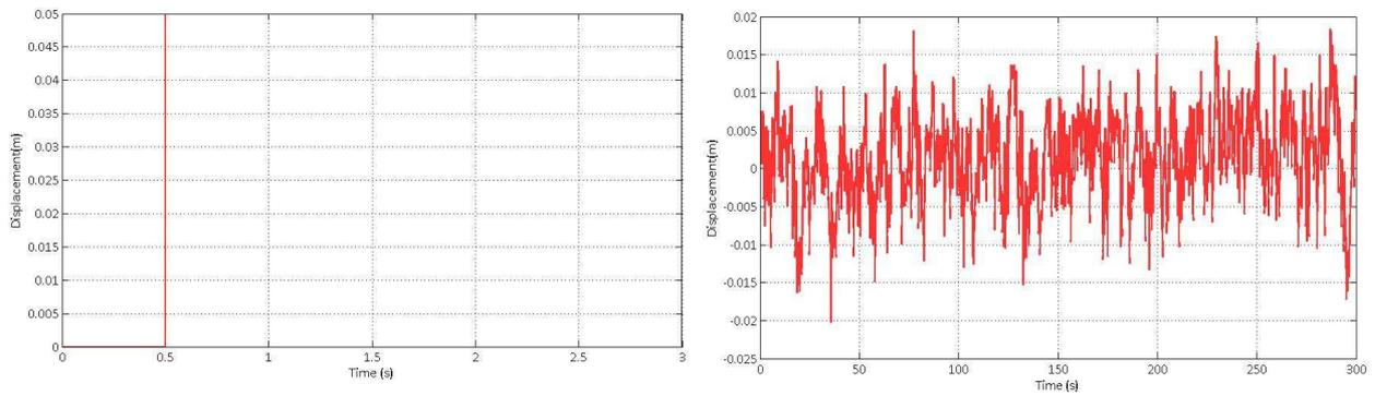
**Figure 2: Input Road Disturbances Modeled as Discrete and Random Events**
