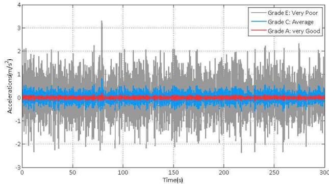
**Figure 11: QFRCo Sprung Mass Accelerations: Random: Effect of Road Grades**
