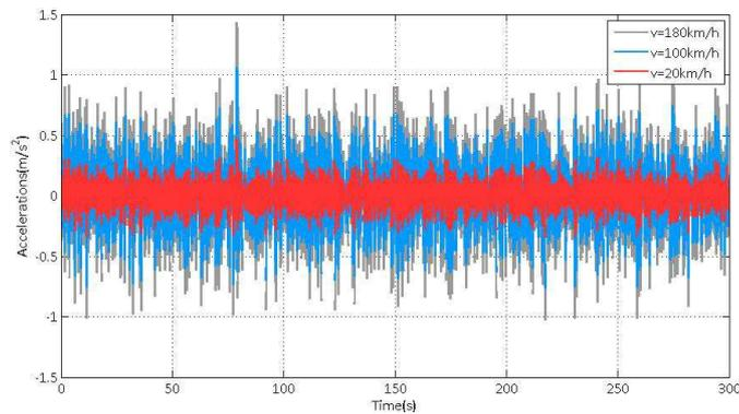
**Figure 12: QFRCo Sprung Mass Accelerations: Random: Effect of Speed**
